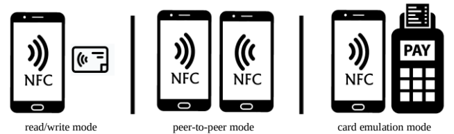
Fig. 1 From left to right, read/write mode, peer-to-peer mode, card emulation mode
