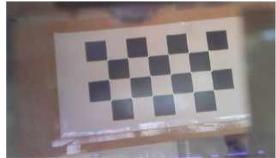
Fig. 14. Viewpoint camera view through the OST display that highlights that the virtual spots (small cyan coloured circles) are perfectly aligned with the inner corners of the real checkerboard. This view also enables the one-time calibration refinement of the parameters of the virtual rendering camera that account for the contribution of the external magnifier.
