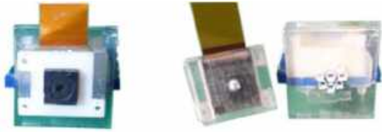
Fig. 15. Viewpoint camera (left) and its holder (right) used to adjust the camera in nine pre-set positions within the eye-box of the optical see-through display.
