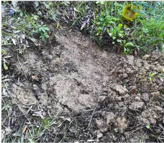
Fig. 3. Compacted soil surface after node burial for the preliminary test.
