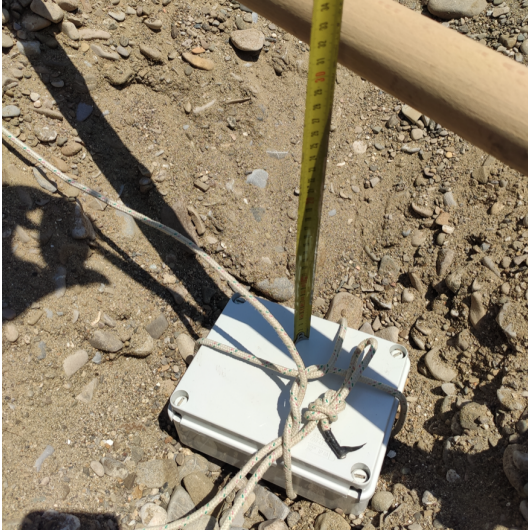
Fig. 6. The IoUT sensor node during tests. Ropes were used to ease the node retrieval.
