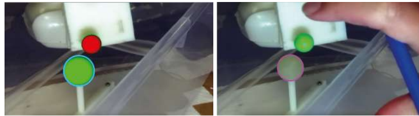
Figure 7. Example of image processing for detecting real and virtual spheres. On the (left), the AR image: the real scene is augmented with the virtual sphere (in green) registered over the lollipop's head and the tracked optical frame (in red). The detected virtual sphere is represented by a blue circle. On the (right), the real image: the detected real lollipop's head is represented by a magenta circle.
