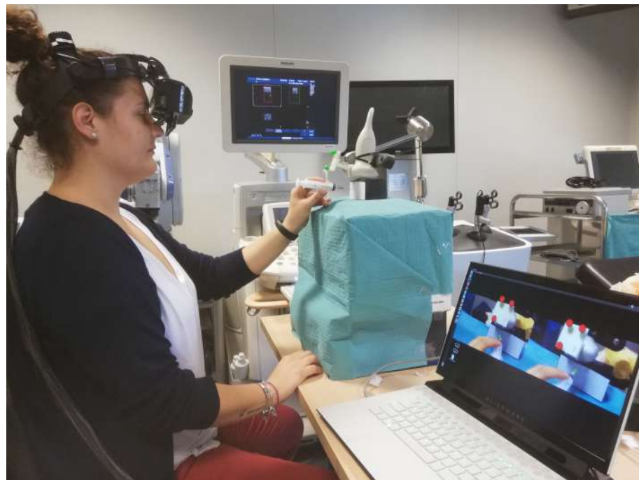
Figure 11. Experimental setup with a user while performing the biopsy task. In the lower right corner are the augmented images projected onto the displays, whereas, on the Philips machine monitor, the real-time ultrasound acquisition can be seen.
