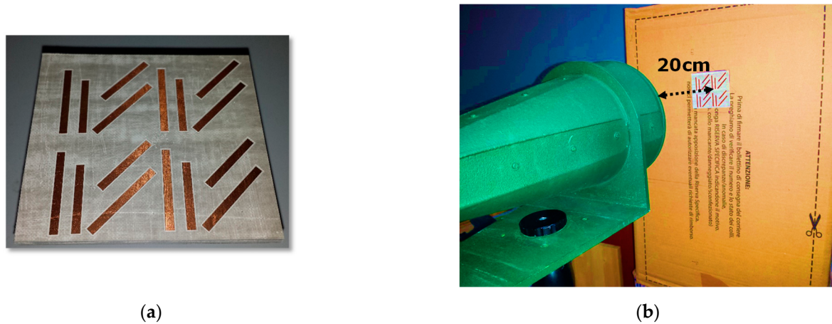
Figure 11. (a) Fabricated prototype of the dual band polarization converter; (b) measurements setup.
