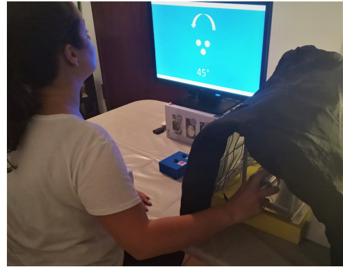
Fig. 3: Participant grasping the knob while reading the rotation to be performed (i.e. 45^\circ counterclockwise).
