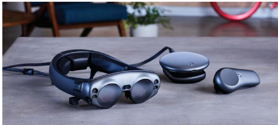
Figure 5. Magic Leap 1 hardware. From left to right: lightwear, lightpack, and control.
