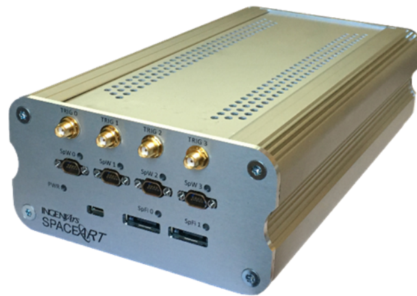
Figure 4. IngeniArs SpaceART Electrical Ground Support Equipment (EGSE) hardware unit.
