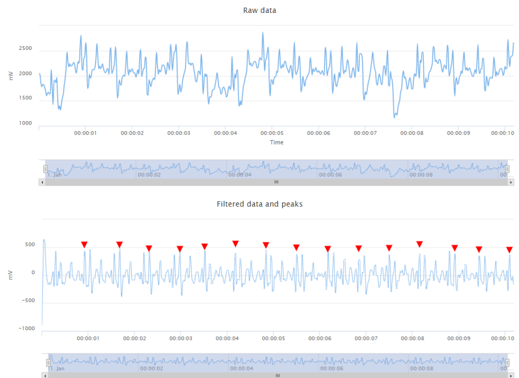
Figure 5. Comparison of raw (top) and filtered (bottom) signal under moderate motion conditions.
