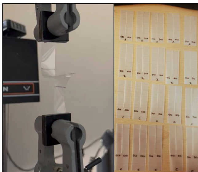
Fig. 2. Film specimens in trouser tear test configuration.
