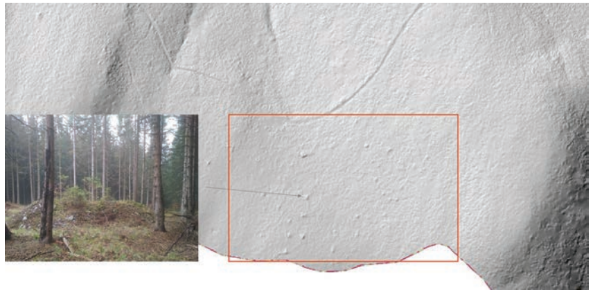
Figure 8. Stone pile—demonstration in the field and in the DRM, elements can be observed in the red frame; ZABAGED®Height chart DMR G5 (ags.cuzk.cz); adjusted.
