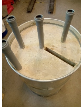
Fig. 13: Realization of the active mock-up with a 2.5 cm lateral slot and several holes to accommodate radioactive sources.
