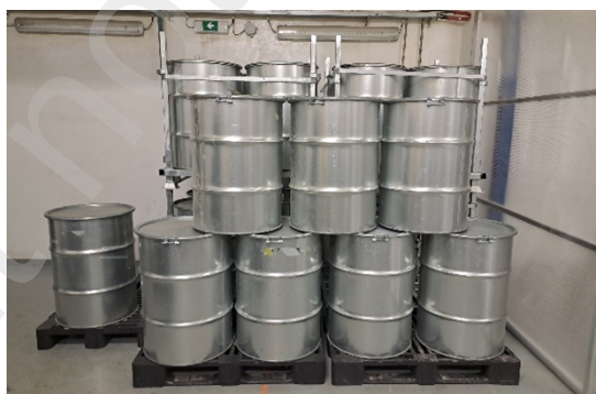
Fig. 12: Configuration used during the demonstration test, with an extra layer of drums placed on top of the inspected mock-ups.
