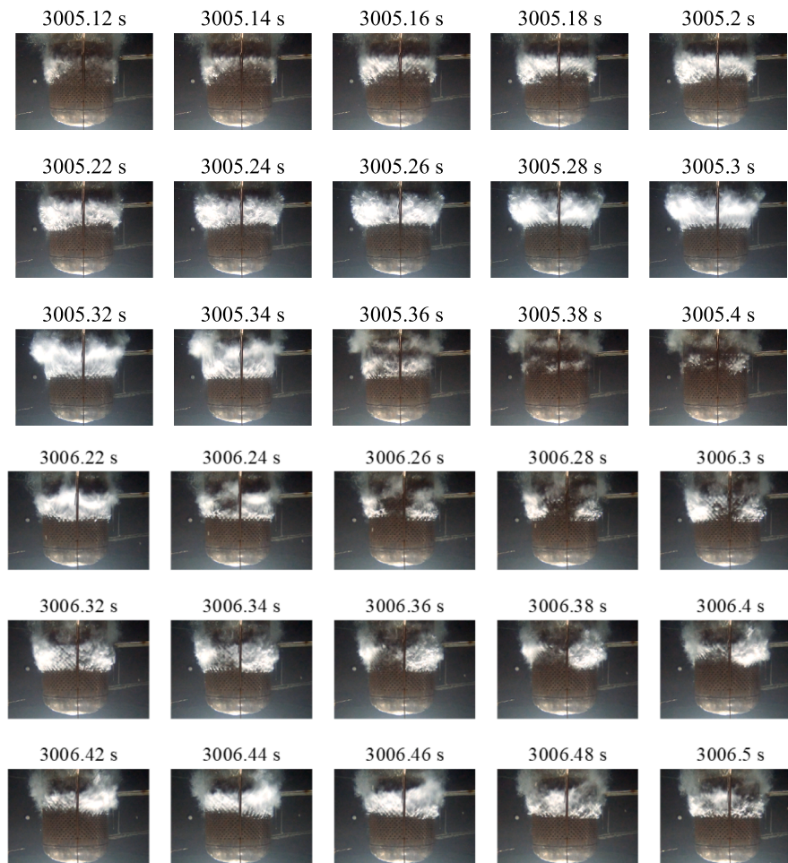
Fig. 14. Bubble dynamics (point G_1 ) when a_{max} + 10\% is beyond r_2 in the region TCC.
