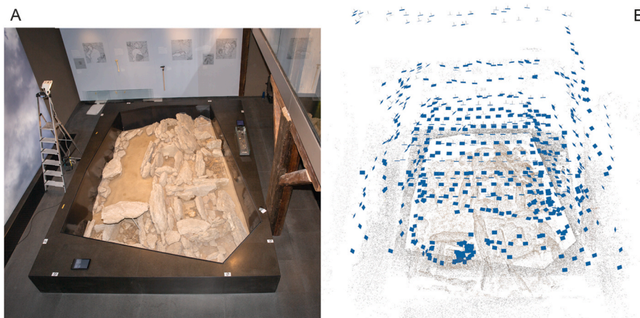
Fig. 5. A) Top view of the funerary monument via the walkway on the upper floor of the Museum Burghalde Lenzburg, B) Point cloud reconstruction and individual camera angles of the funerary monument displayed in Metashape Professional (Agisoft LLC, 2021).
