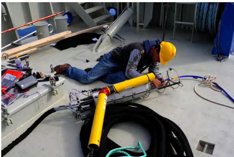
Figure 6: STU during a communication test on Gunnurus deck before deployment. The two yellow cylinders are the KM modems, of which, one is the STU’s and the other is for testing. The grey box contains the STU electronics. It is also visible, in the photo, the blue cable used to connect the STU to shore, the black thermistor chain and the hydrophone array.
