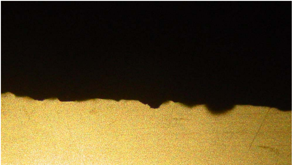
Figure 8. Profile of a new electroplated tapered diamond bead (top). After cutting for 1 hour (bottom), most diamond grains are still in place but they appear blunt (no breakage).
