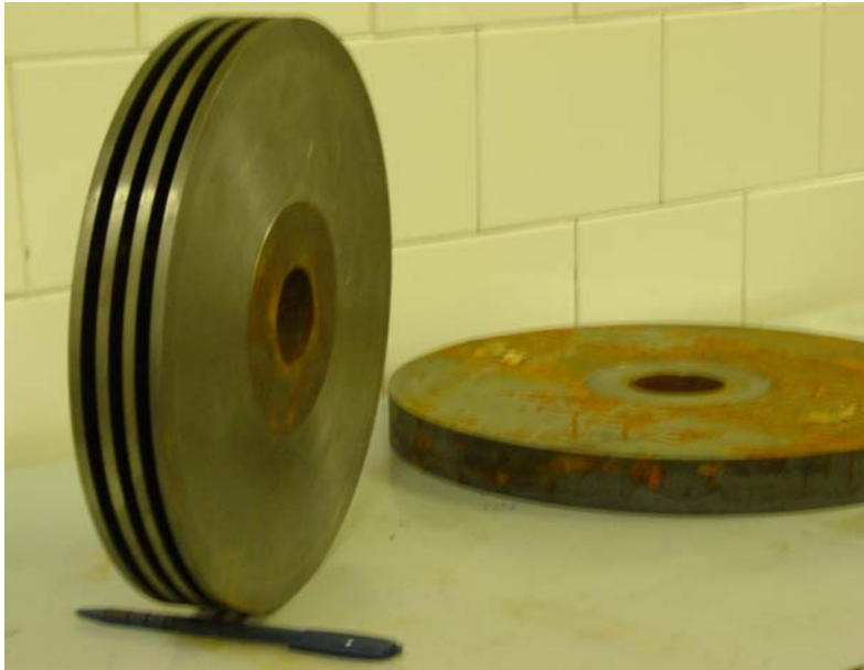
Figure 3. A new cast iron disk with three grooves (left) and before preparation (right). The axial hole is for mounting on the testing machine.
