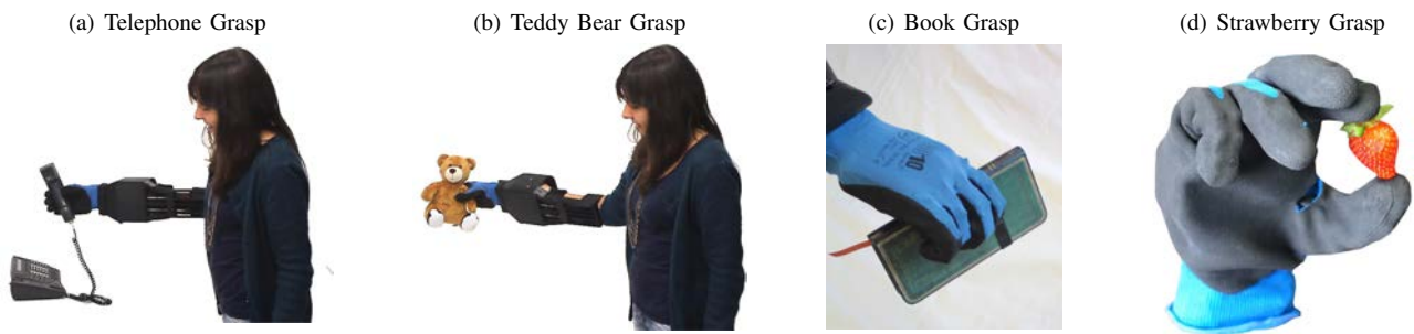
Fig. 23. Some examples of grasps executed with the robotic hand mounted on a wearable Human Interface: telephone (a), Teddy Bear (b), book (c), and strawberry (d)
