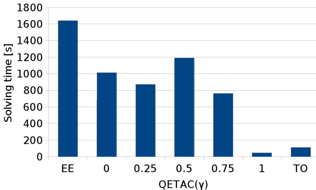
Fig. 8. Solving times as a function of the  $\gamma$  value.
