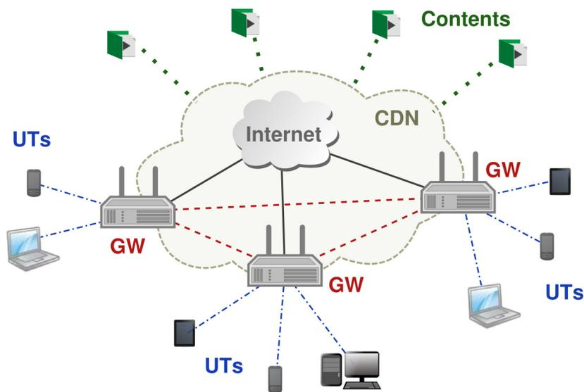
Fig. 1. Architecture of the CDWMN. Solid lines represent wired links, dashed lines wireless links, and dotted lines (towards the contents) virtual links.
