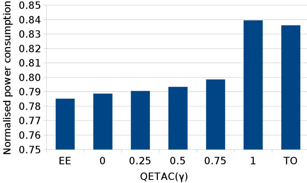
Fig. 4. Normalised power consumption of QETAC as a function of the  $\gamma$  value. Lower is better.
