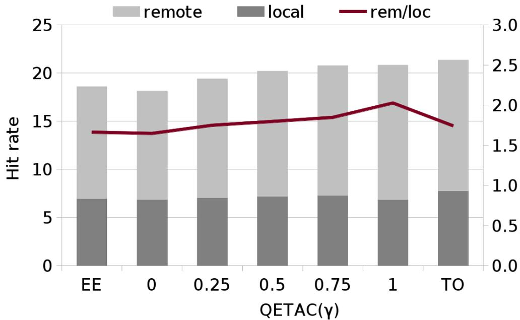
Fig. 7. Local and remote hit rates (stacked bars) plus remote/local hit rate ratio, as a function of the  $\gamma$  value.
