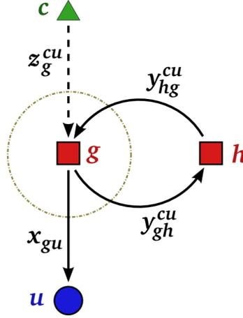
Fig. 2. Depiction of the flow conservation constraints (5). The same figure applies to (6) by removing user  $u$ , the  $(g, u)$  link, and the  $x_{gu}$  variable.
