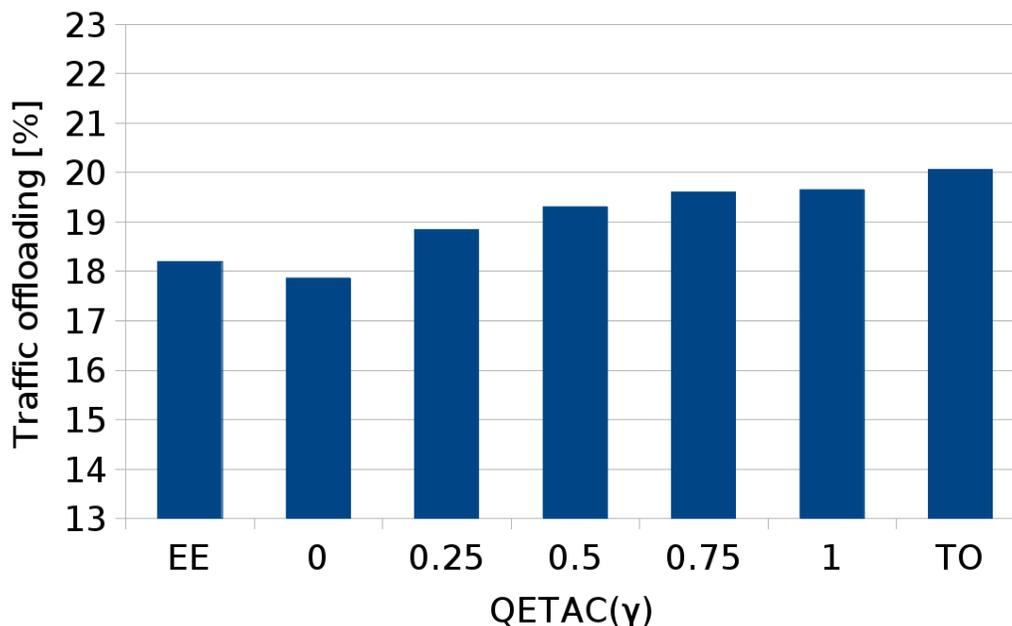
Fig. 5. Percentage of traffic offloading as a function of the  $\gamma$  value. Higher is better.
