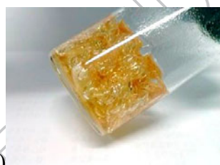
Figure 4. a) Cross-linked insoluble polymer obtained by reacting 1 g of L-DOPA with 1.644 g of CDI in 4 ml of anhydrous DMF at room temperature. The gelation point was reached after 1 day. b) HPLC analyses of L-DOPA. On the left: standard L-DOPA solution; on the right: L-DOPA extracted from MIP(1:4)+10% L-DOPA.
