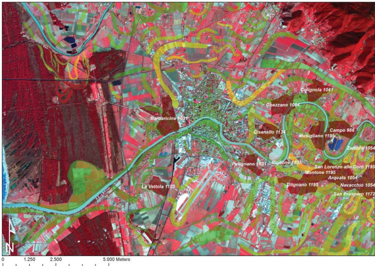
Fig. 2.12 The traces of the possible paleochannels (from red to green according to the trace's level of reliability, from BINI et alii 2012a), associated with the toponyms where the Arno is attested.
