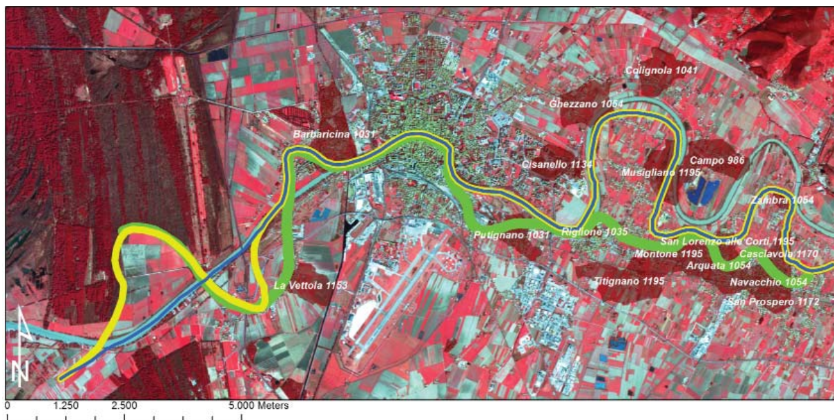
Fig. 2.13 Reconstruction of the possible courses of the Arno River during the Early Middle Ages (green) and Late Middle Ages before (yellow) and after the cut of the meanders of La Vettola and San Rossore (dark blue). The areas of the toponyms with the date of the first attestation of passage of the Auser River are in brown.
