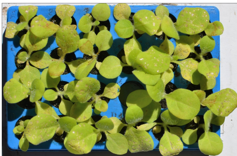
Figure 5.8 – The miniaturized kit for biomonitoring of O_3 with tobacco Bel-W3 seedlings. The external dimensions are 12.5x8.5 cm. Please note necrotic lesions induced by the exposure to ambient air in the presence of O_3 .
