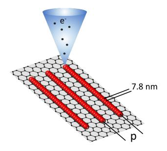
**Figure 1.** Sketch of the electron irradiation: red spots indicate the landing points of the primary e-beam. All lines are exposed with a step size of 7.8 nm (distance between the landing points) and are separated by a distance *p*.
