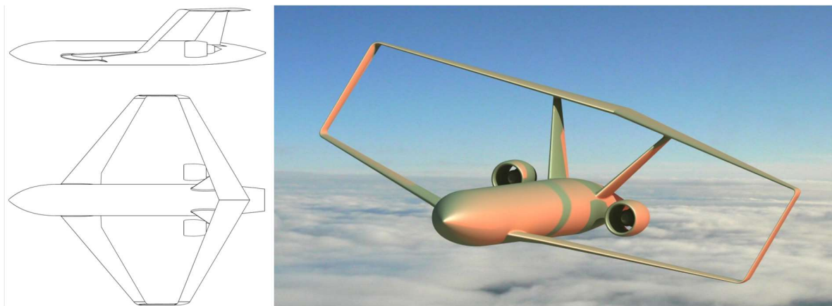
Fig. 10 Views of the medium range PrP object of study in the project "PARSIFAL"
