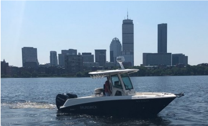
Figure 2. R/V Philos (RoboWhaler). RoboWhaler is an autonomous surface vessel that is used for advanced autonomy and sensor fusion algorithm development.
