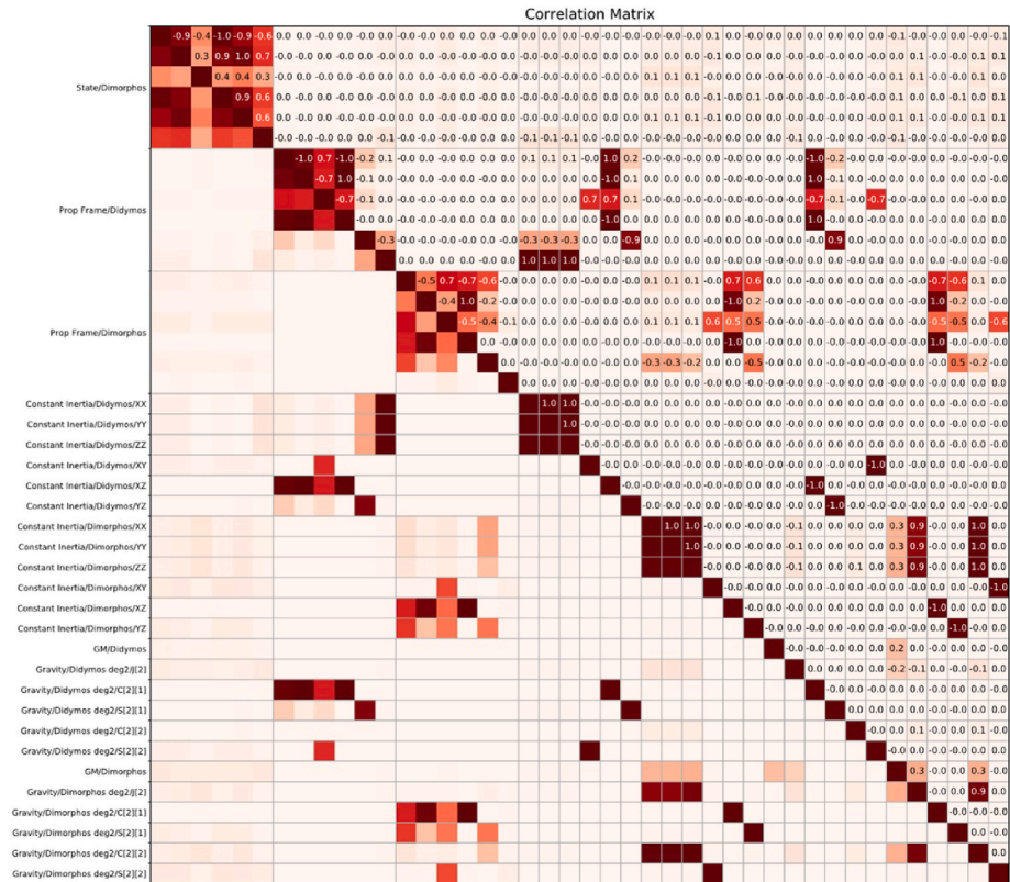
Fig. 32. Correlation matrix of the F2BP pre-impact relaxed simulation for the main parameters of interest. For clarity, some parameters in the correlation matrices are grouped: the state of Dimorphos parameters includes [X, Y, Z, DX, DY, DZ], the F2BP propagated frame comprises [RA, DEC, W, \omega_X , \omega_Y , \omega_Z ].
