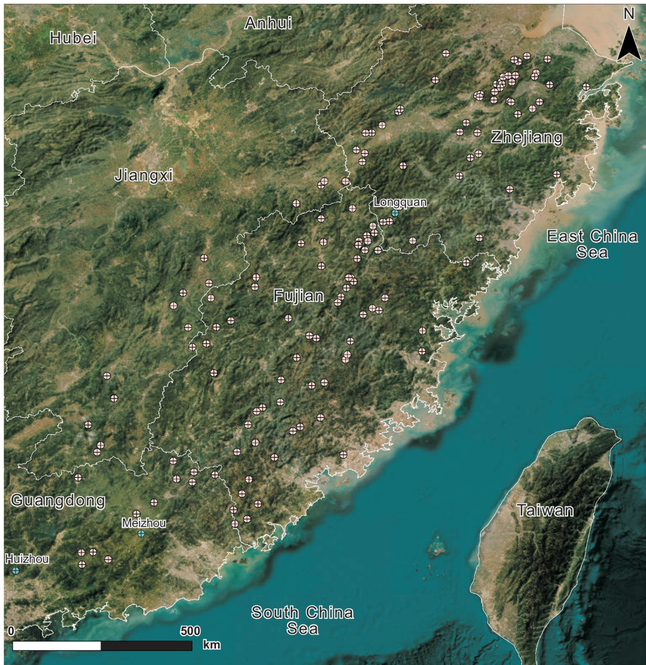
Figure 5. Satellite image of coastal southeastern China. The pink circles indicate sites where the presence of fractured bedrock is likely due to the morphological, lithological, and climatic similarities with Longquan site. Longquan, Huizhou, and Meizhou sites where mineral water exploitation is already active are marked using cyan circles.
