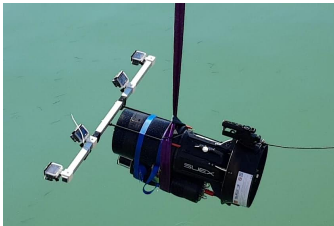
Figure 1 - SDS employed during the mission, acoustic transponder below the scooter, cameras on the left (Costanzi et al., 2019).
