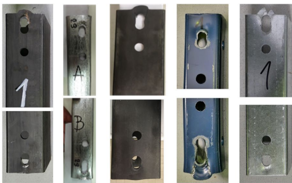
Fig. 13 Local tests: a Force-displacement curves (solid lines) versus code predictions accounting for actual material strength (dashed lines), and b damaged configuration under tensile load (T)
