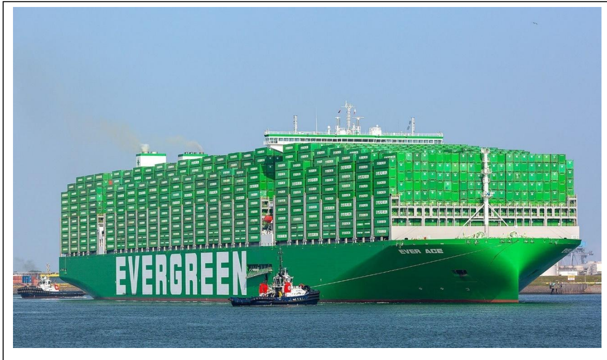
Figure 1. Flattened vertical bow of "EVER ACE" (EVERGREEN, 2021)
