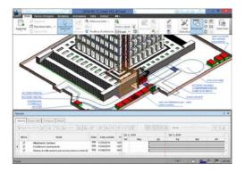
A BIM-based site plan can be used to produce illustrative representations of the site and safety arrangements, and the views can be used for orientation of site workers, task guidance and instructions, for informing about risks.
