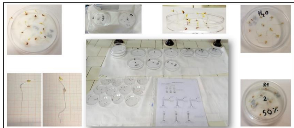
Figure 2. Set-up of the L. sativum seed germination test and germinated seeds after 72 h.
