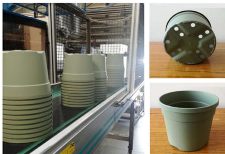
Figure 8. Injection molding pots of Matrix1_30 formulations.
