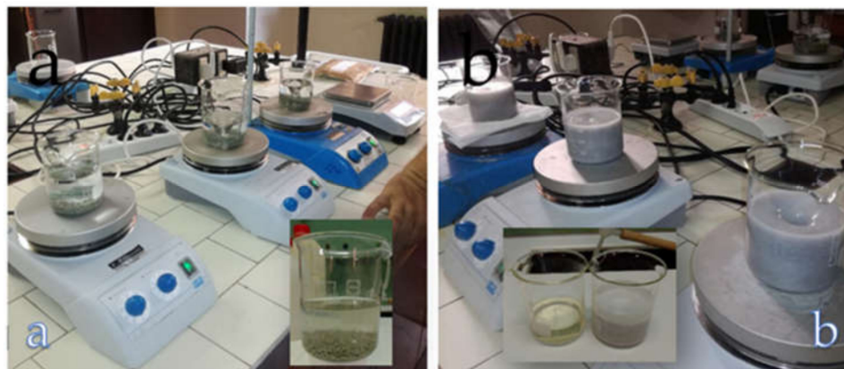
Figure 9. (a) Set-up for the preparation of the eluates and (b) the eluates obtained from PS and graules containing 30 wt.% PS (Matrix1_30).
