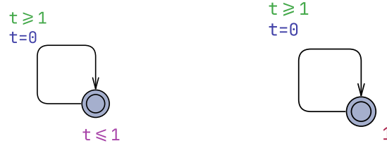
Fig. 7: Simulation automaton to control enabling transitions. On the left with a constant exact transition time of 1s and on the right with an exponential distribution of transition times with \lambda = 1 .
