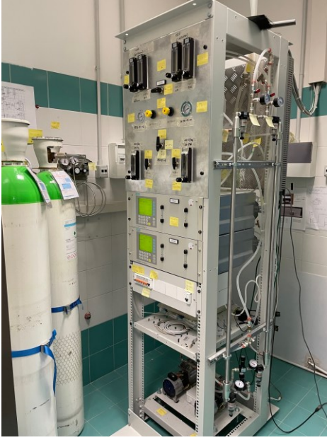
Figure 5. Instrumentation rack hosting the gas analyzers.
