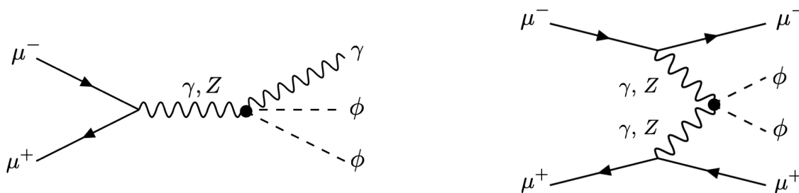
Figure 6. Representative Feynman diagrams for DY-like (left) and neutral VBS-like (right) pair-production of scalar \phi particles through the operator of eq. (2.1).
