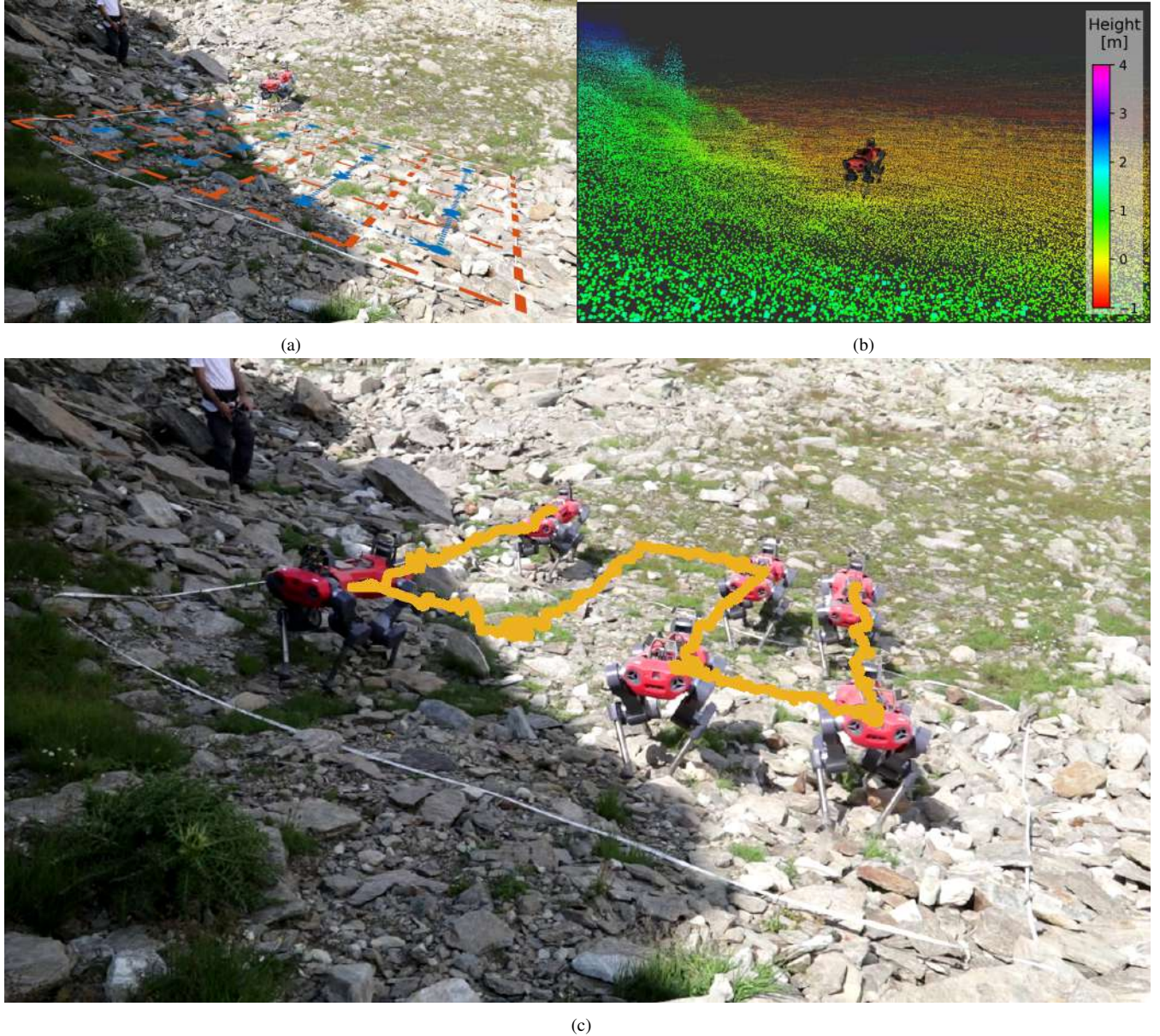
FIGURE 8: (a) NI 1 plot with the square grid (in orange) and the waypoint trajectory (in blue) superimposed on the image. (b) Point cloud of the surroundings obtained with the lidar during the mapping phase. The color of the points indicates their height. (c) Overlapped snapshots and actual trajectory (in yellow) of ANYmal performing a monitoring mission. The corresponding video is available in the supplementary material.
