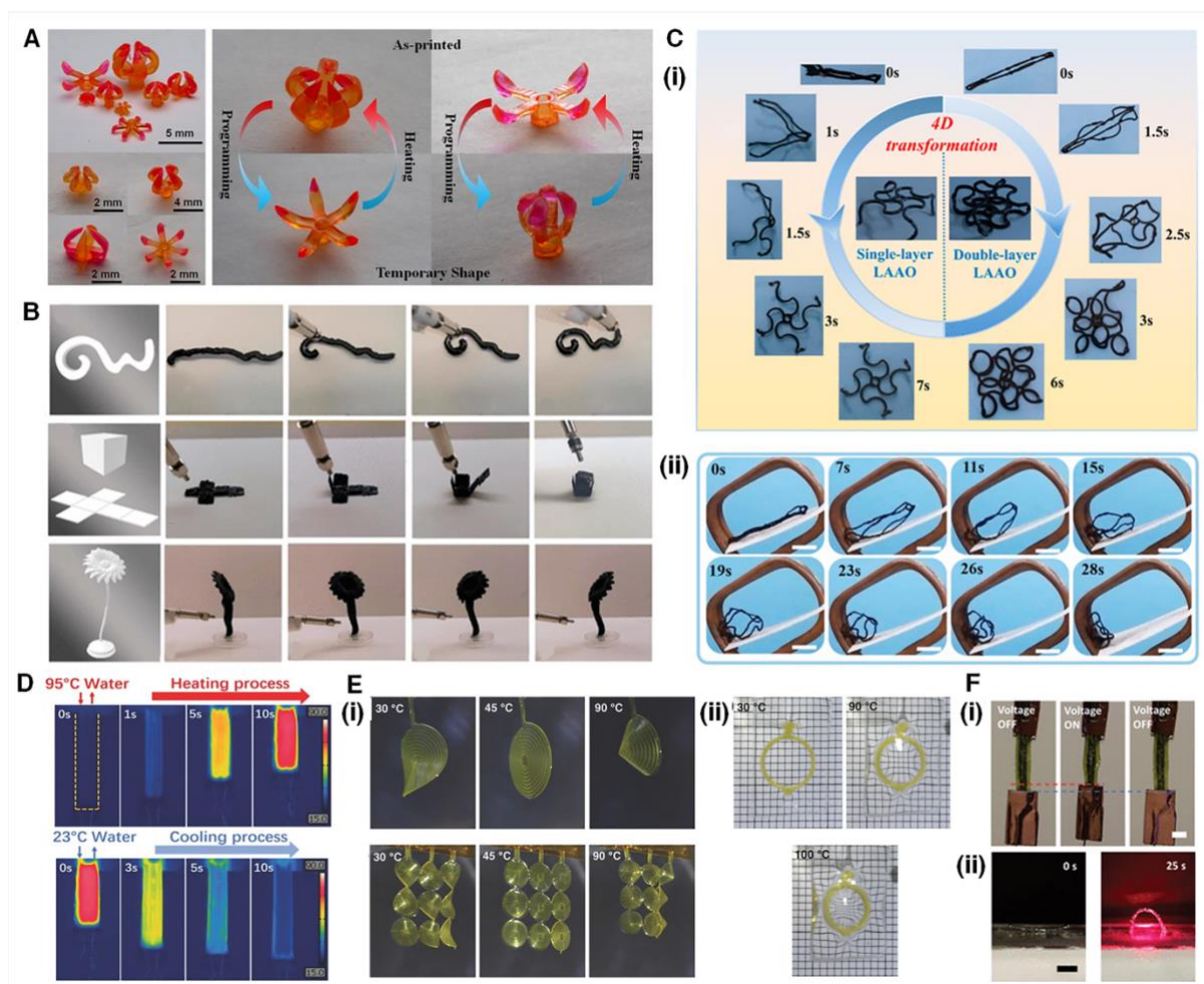
Figure 2 Relevant examples of SMMs in 4D printing technology. (A) Photo images of the fabricated 4D grippers with different designs and shape transformation. Reproduced from 43 with permission from Springer Nature. (B) Photo images of sequential shape changes of the 4D printed constructs under the NIR exposure. Reproduced from 75 with permission from American Chemical Society. (C) Photo images of (i) thermo-responsive and (ii) magnetic-responsive 4D shape change steps of single and double-layer left atrial appendage occlude (LAAO) constructs. Reproduced from 64 with permission from American Chemical Society. (D) A thermal image of an LCE-based artificial vascular muscle during heating (contraction) and cooling (relaxation) processes. Reproduced from 117 with permission from John Wiley and Sons. (E) Sequential photo images of (i) 4D LCE single (diameter = 8 mm) and multiple spiral (diameter = 5 mm) architectures and (ii) 4D lens property change (grid = 2.5 cm) in response to temperature variation. Reproduced from 120 with permission from John Wiley and Sons. (F) Sequential photo images of the 4D LCE actuator, leading to shape change in response to (i) electro-thermal (shrinkage/expansion) and (ii) NIR-based photo-thermal (structure bending) stimuli. Reproduced from 67 with permission from American Chemical Society.
