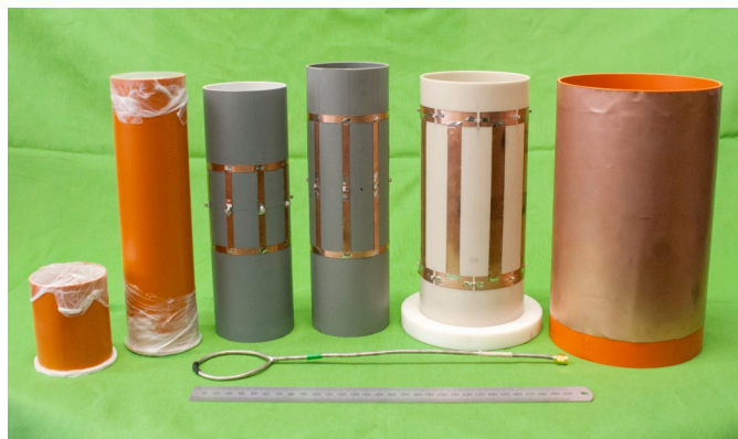
Fig. 2. Nested DT RF birdcage coil prototypes suitable for 2.35 T applications (geometrical details in section II.D). Left to right: short and long samples; short and long ^{23}\text{Na} LP; ^1\text{H} HP; and RF shield. The coupling loop is also shown.
