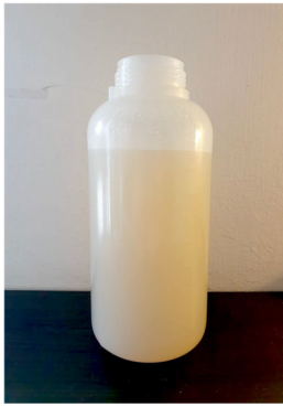
Fig. 15. Realized biological phantom: a plastic bottle filled with a solution of water, agar, and NaCl used to simulate the brain tissue.
