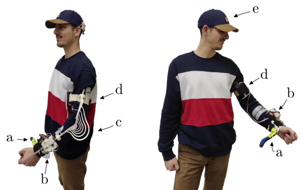
Fig. 1. The Robotic Sixth Finger (a) and its power supply and control system (b) developed by US has been integrated with the Assistive Elbow Orthosis (c) developed by UT and the CUFF (d) from UP. The CUFF has been modified to be completely wearable. Motion of the finger is controlled by a new e-Cap version (e) developed by US with novel 3D-printed electrodes by UT
