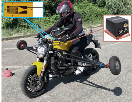
Figure 1. The instrumented motorcycle with outriggers, as used in the experiment. The positions of the inertial platform and strain gauges are shown.
