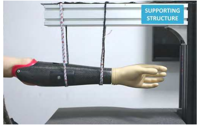
Fig. 3: Tactile Feedback Perception Experiment setup: the prosthetic limb (here with VP hand) is kept in place by a supporting structure made of beams and two cables with Velcro.
