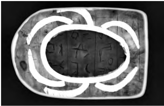
Figure 9.11. X-radiographic image of heart-scarab EA7876 produced using a Siefert DS1 X-ray tube operating at 100 kV with an exposure of 5 mA for four minutes.
