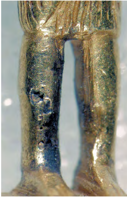
Figure 9.21. Details of one of the amulets representing the standing figure of god Seth (E7715): (left) defects on the right leg due to improper casting (shrinkage and gas cavities); (right) chased motif with tool marks corresponding to engraving perhaps from a modern restoration.
