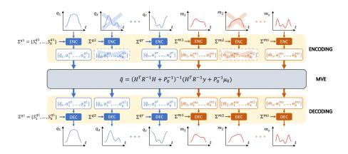
**Figure 1.** Schematic flow of the estimation procedure. First temporal signals are mapped on the weight vector through the fPC bases (*Encoding*). After that, *Minimum Variance Estimation* (MVE) fuses the encoded measures with *a priori* knowledge to estimate for the missing part of measures. In the end, the estimated weight vector is converted back to the temporal domain (*Decoding*).
