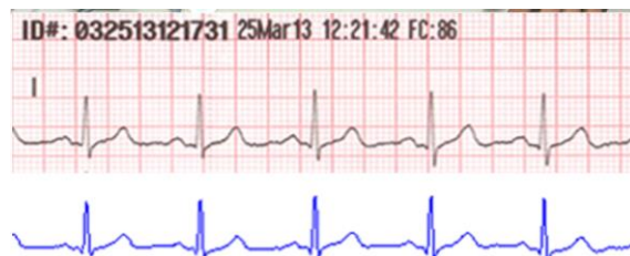
Fig. 5. Comparison of the ECG acquired using Lifepak and the prototype
