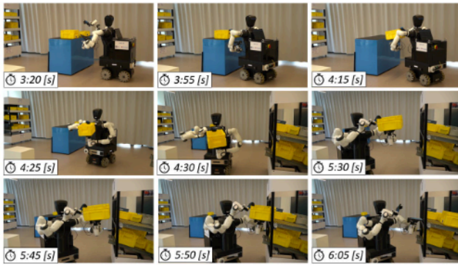
Fig. 4: Testing of the autonomous framework for logistics. Reading from left to right, up to down, we report a photo sequence of the box picking from the support, followed by the robot autonomous navigation and box deposit on the machine side.
