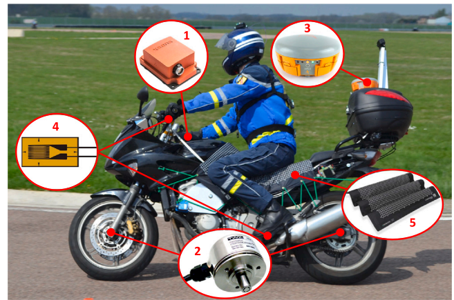
Fig. 2. The instrumented motorcycle. The annotations show each sensor's placement.
