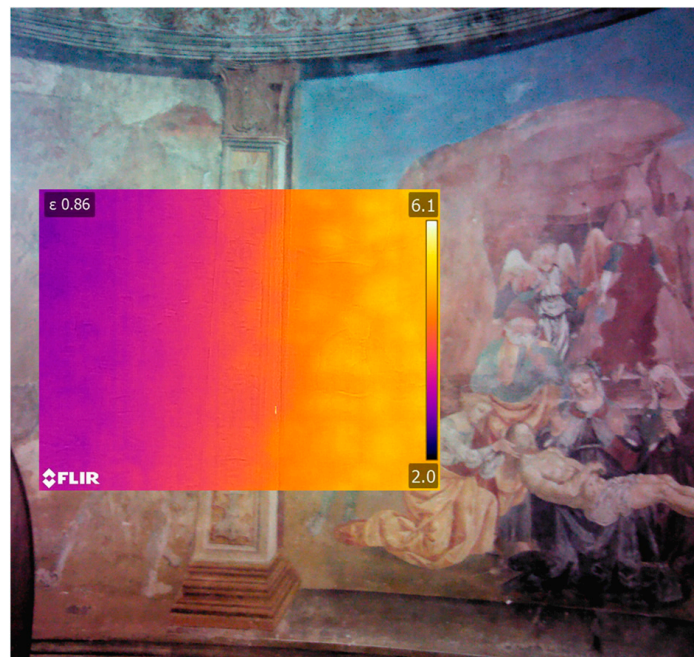
Figure 4. Passive IRT image of the attachment point of panels A and B. An abrupt discontinuity in the average emitted radiation can be seen.
