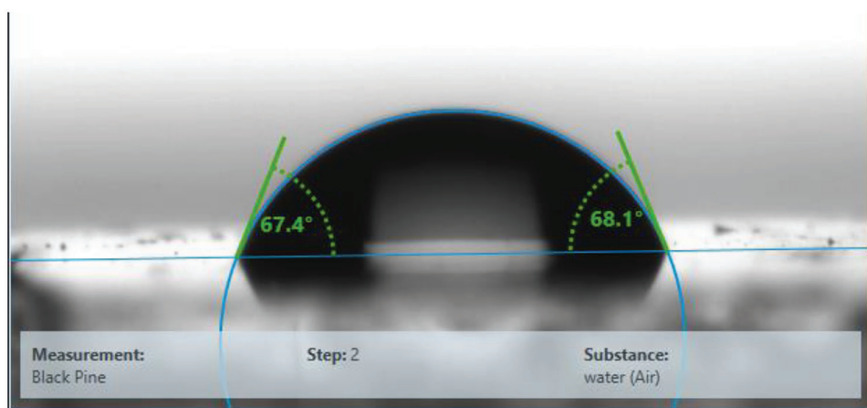
Figure 7. Contact angle of black pine resin. Left angle (water): 67.4^\circ ; Right angle (water): 68.1^\circ . Total surface energy, 49.1 \text{ mN m}^{-1} with a polar component of 6.9 \text{ mN m}^{-1} and disperse component of 42.2 \text{ mN m}^{-1} .
