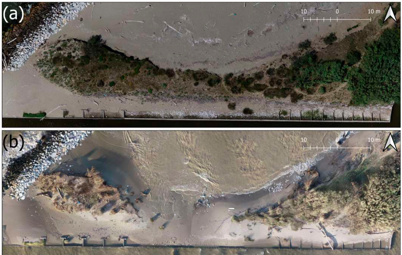
Figure 12. Orthomosaics acquired in June 2023 (a) and November 2023 (b) showing the dismantling of the dune system at the southern end of the study area. The breach led to direct contact between seawater and the drainage canal of the reclamation system, compromising the separation between marine and inland waters.
