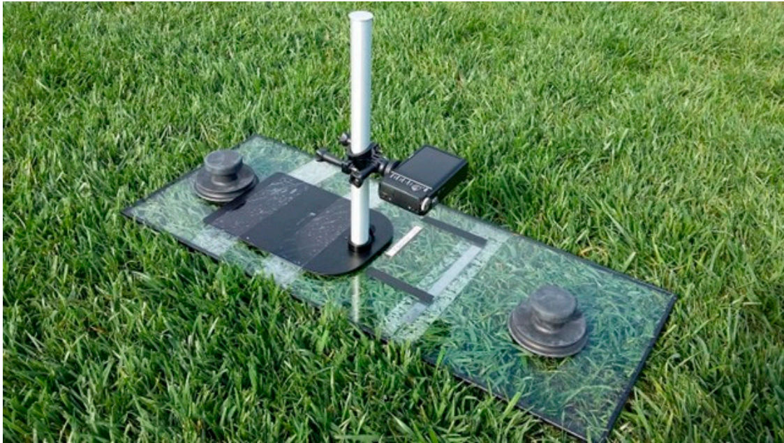
Figure 4. Cleanness of cut prototype instrument.
